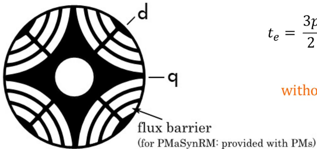
$$t_e = \frac{3p}{2} (\underbrace{\psi_{PM} i_q}_{\text{without magnets } \psi_{PM} = 0} + (L_d - L_q) i_d i_q)$$
