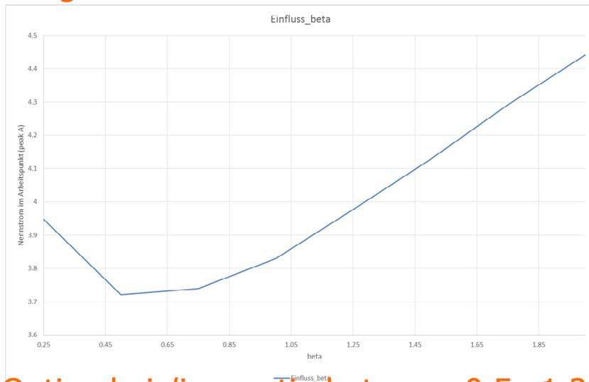
Optimal air/iron ratio between 0,5...1,25
